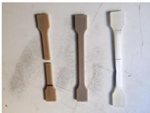
CNF mixed Plastic test pieces
