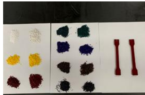
left: PLA+ color pigment right : PLA + color pigment + nano cellulose
